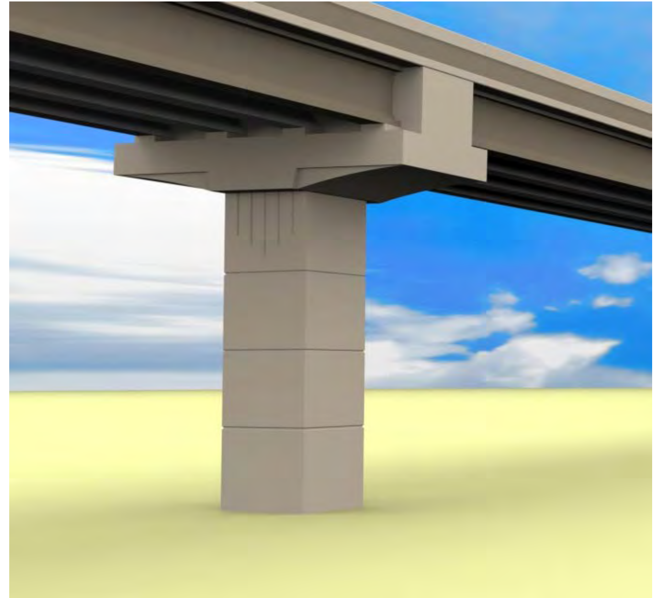
Inverted "T" - Symmetrical Hammer Head – Single Structure
