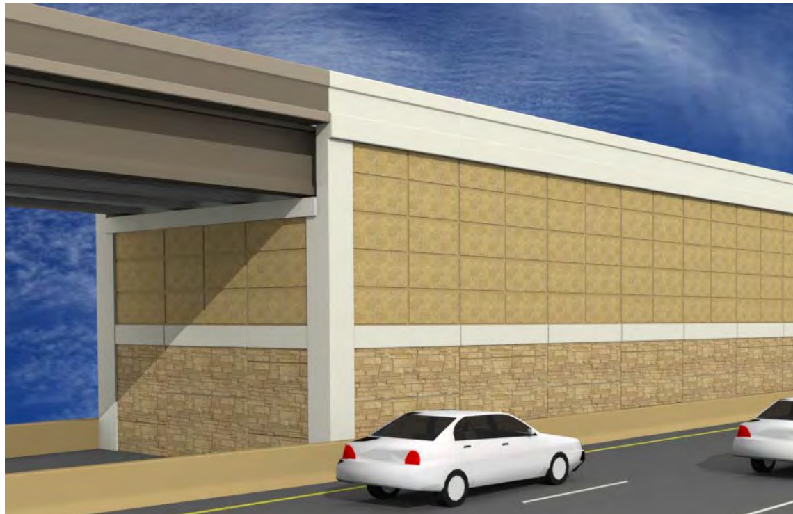
Loop 1 Aesthetic – Vertical Abutment at DC to US 183 N
