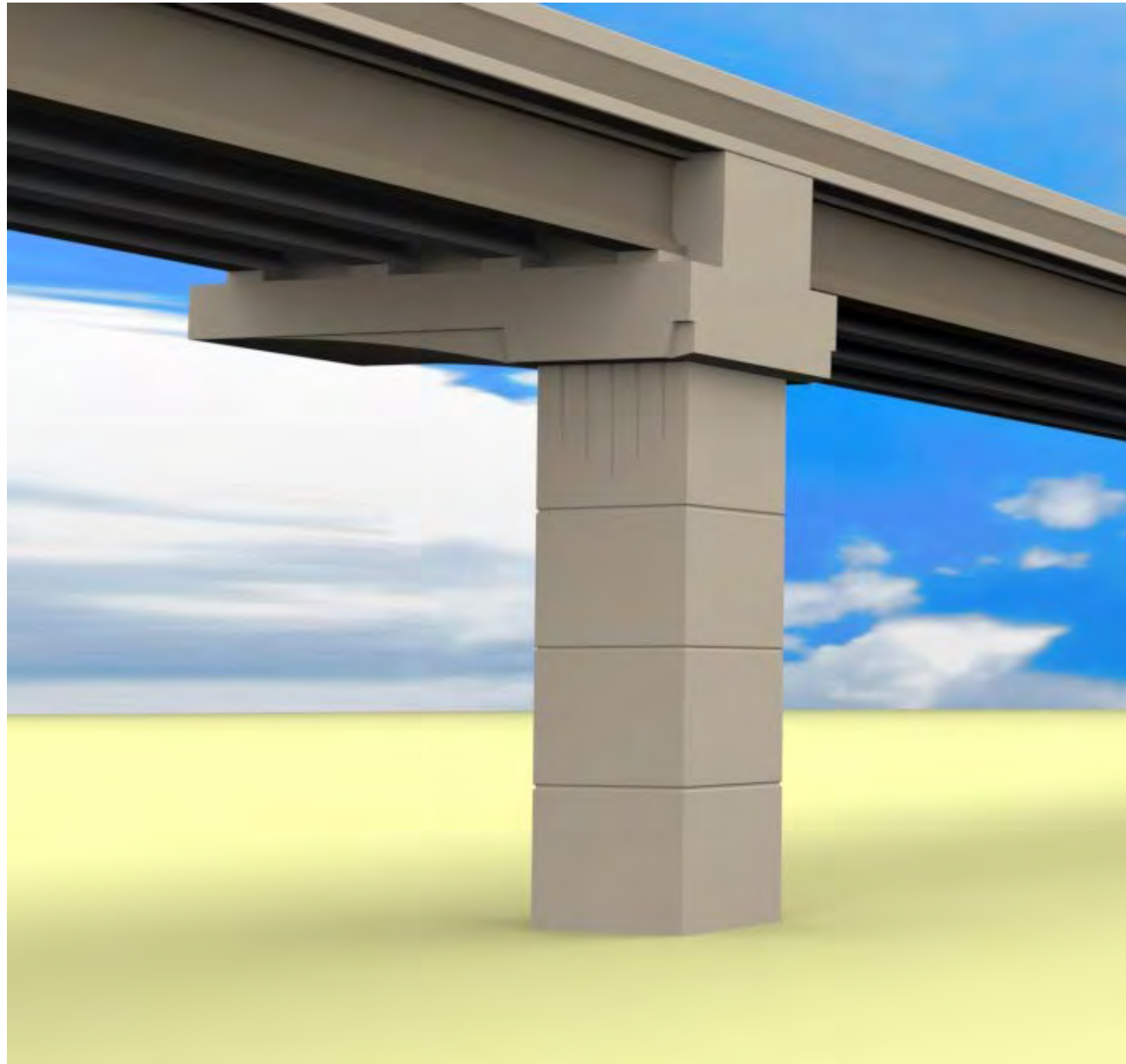
Inverted "T" - Cantilever Hammer Head – Single Structure
