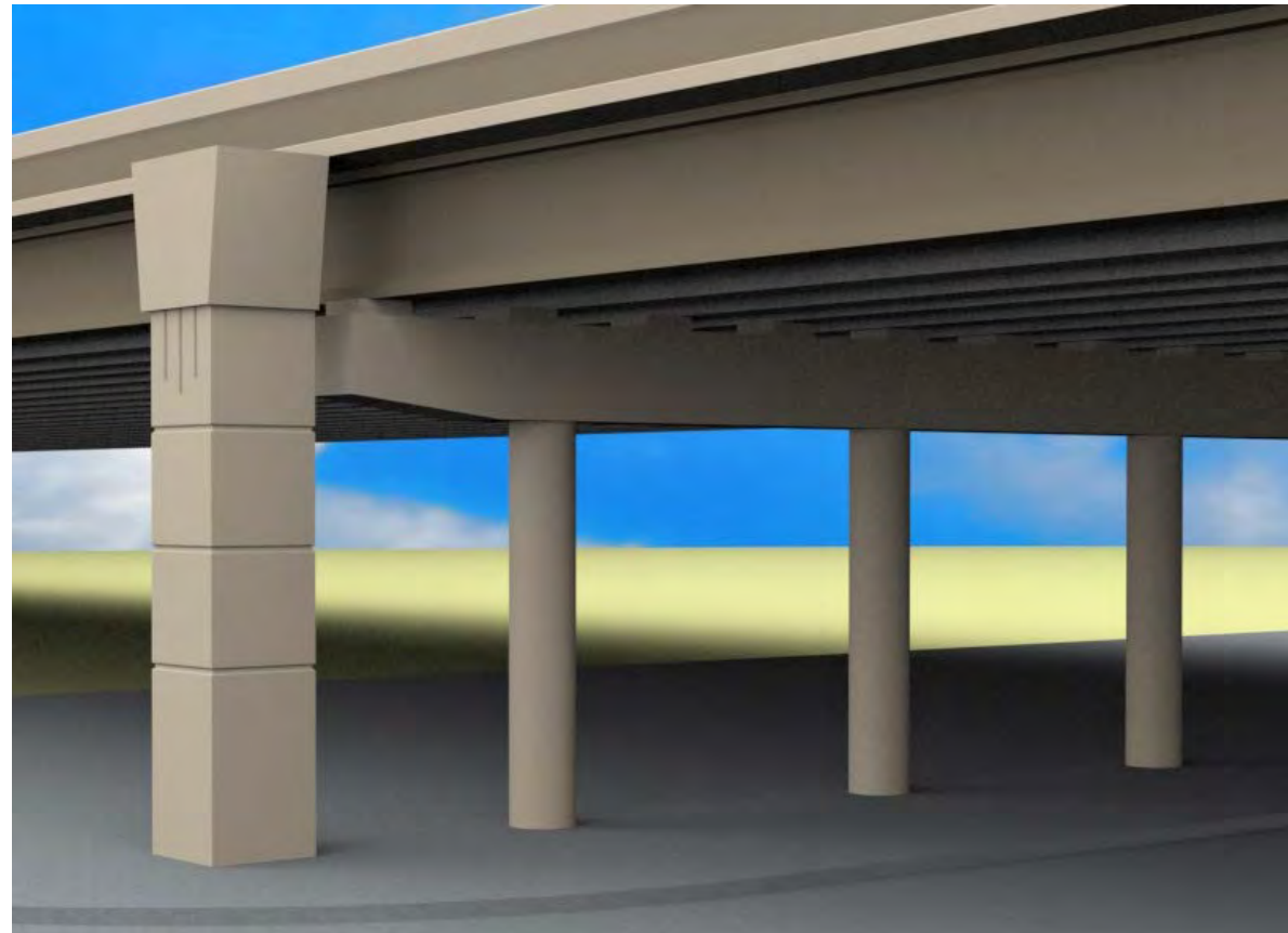
Exterior Decorative Column in-line and outboard of existing bent line where no outside widening of Structure. Existing interior cylindrical columns remain
